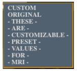
The **Preset** Menu for MRI, shown left, allows for 7 programmable preset names and values that can be assigned.
