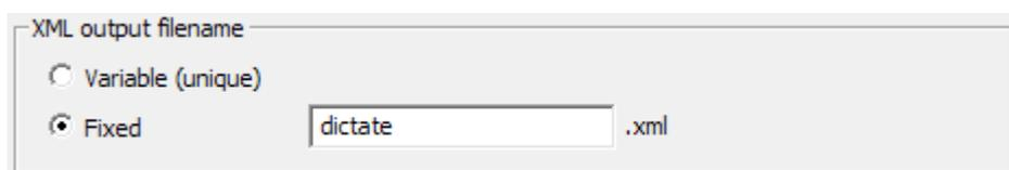
In "Fixed" mode, the filename has to be defined without extension. FUSION will automatically add the extension ".xml". The filename "fusion" (case insensitive) is reserved and cannot be used.
